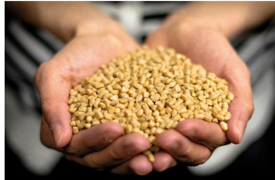
One of the several ways to reduce the CO2 footprint of a product is to use a biocomposite. Here, you can see a granulate made of PP (polypropylene) and wood fibers.
